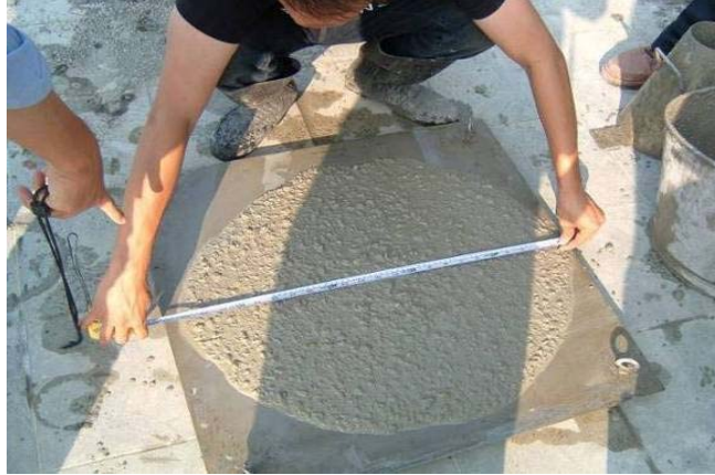
Figure 23 Photo of self-compact concrete, high slump
